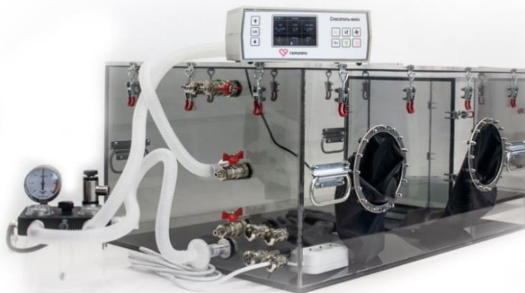
Figure 1. View of the gas exchange chamber for rodents.
